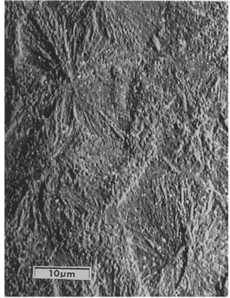
Fig. 6. Spherulites in the core zone of an injection moulding of PP containing 10% w/w of pigment. Pigment particles (white) can be seen within the spherulites (SEM micrograph of etched cut surface).
